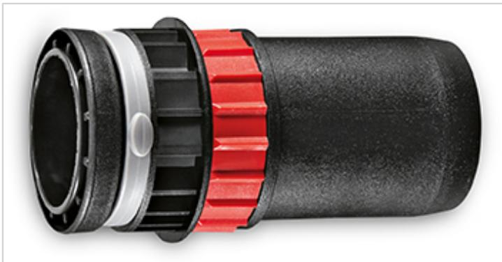
For connecting a FLEX power tool to extraction units from other manufacturers. Suitable for hoses inside Ø 27 mm, outside Ø 36 mm, with auxiliary air adjustment.
