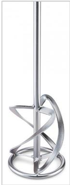
Three clockwise helices screw themselves into the material. This provides fast, intensive mixing of even the heaviest and toughest mixtures, with little effort. Also known as a mortar or tough mixture paddle. Ideal for: mortar, concrete, plaster, screed, plasterboard bonding compound, bitumen coating.
