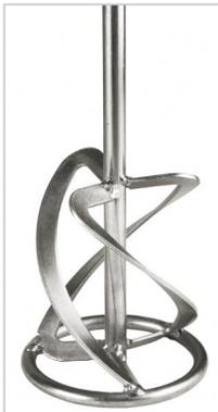
Three anticlockwise helices press down the mix in the container. Any deposited pigments, solids or fibres are forced upwards and evenly mixed. The mix does not splash. Ideal for liquid and creamy mix: paints, emulsion paints, gypsum plaster, casting compounds, fibrous materials.
