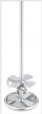
Two discs with counter-running angled blades create a dynamic flow in the mixing container. The blades on the discs force the material being mixed in opposing directions downwards or upwards. Ideal for mixing liquid to tough material: Paint, emulsion, paste, glue, jointing mortar.
