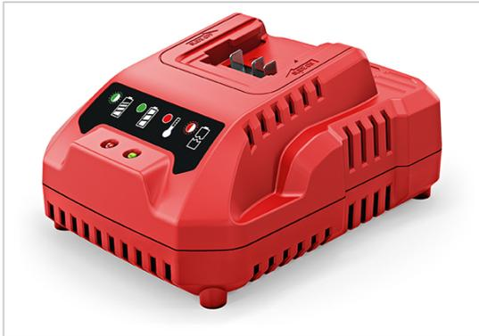
For charging 10.8 V battery packs. With LED charging level indicator, suspension hole, high energy transfer rate and low energy consumption. Charging time approx. 40 min. for 2.5 Ah, approx. 55 min. for 4.0 Ah and approx. 85 min. for 6.0 Ah batteries.
